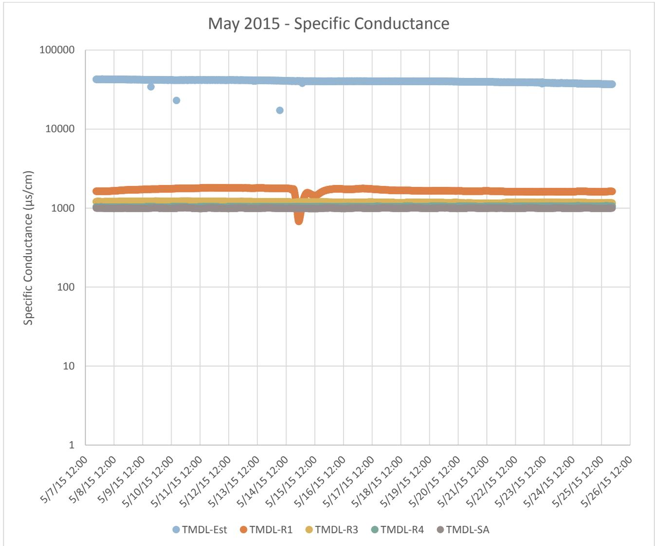
Note: The TMDL-R2 results for specific conductance are highly suspect, as the values decreased noticeably from the time of deployment and dropped well below both the expected range and the values measured by the upstream and downstream sondes. Fouling is suspected. The data is excluded from this chart but is included in the electronic attachments to this report. Specific conductance is not a required continuous monitoring parameter so the sonde was not re-deployed for this quarter.
