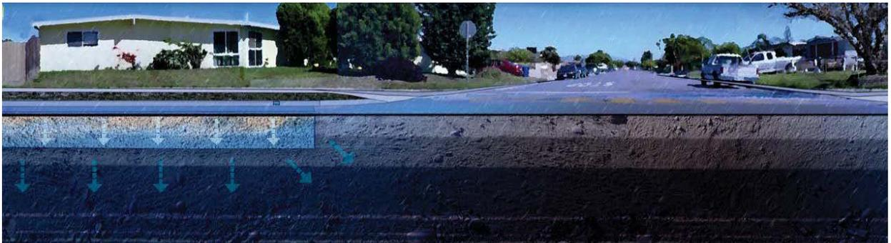
4. Oak Park Green Streets Retrofit project. Approximately 95% project design is to treat about 1,700,000 cubic feet of runoff annually from over 82 acres of residential area in Oak Park. The proposed biofiltration treatment is to meet compliance with Malibu Creek Bacteria TMDL. Construction is scheduled for summer of 2017. Total cost for the awarded project is \$1.75M.
