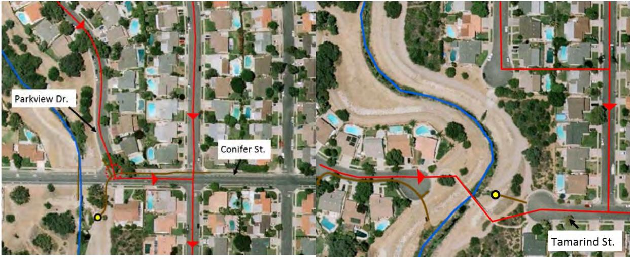
**Fig.2.8. Detail of storm drain (brown) and sanitary sewer (red) infrastructure near M05 (yellow circle, left map) and M02 (yellow circle, right map). Sanitary sewer crossing above storm drain is indicated by dotted red circle.**
