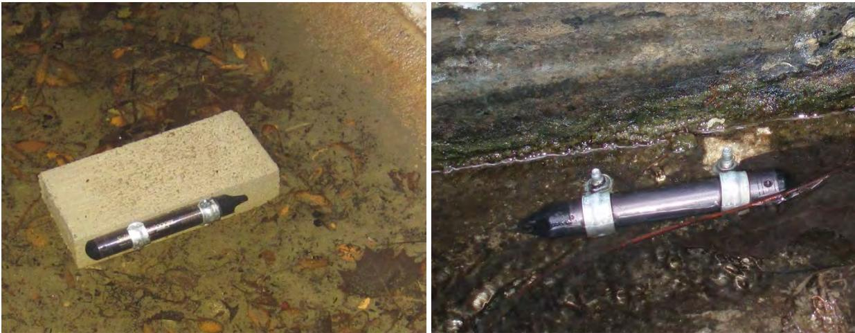
Fig. 3. Deployment of Solinst Levelloggers in storm drains and open channels
