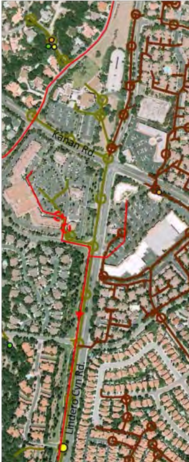
**Fig.3.8. Detail of storm drain with manholes (City: green, County: brown) and sanitary sewer infrastructure (red) near TL3 (large yellow circle). Sanitary sewer crossings above the storm drain are indicated by dotted red circles.**
