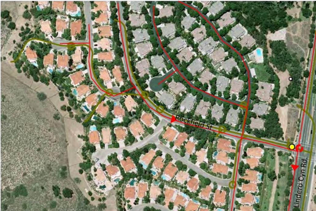
**Fig.3.6. Detail of storm drain with manholes (green) and sanitary sewer infrastructure (red) near TL2 (yellow circle). Sanitary sewer crossing above the storm drain is indicated by dotted red circle.**
