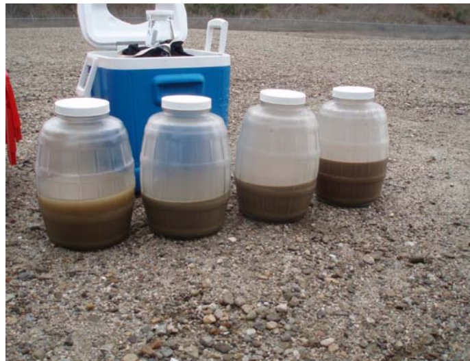
Figure 15: Wet weather composite sample collected at Mass Emission Station ME-SCR during December 2007 showing high suspended solids content
