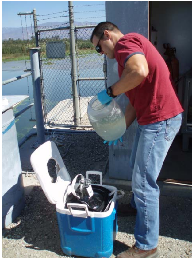
Figure 14: Composite Sample Collection using EPA Sampling Protocols
