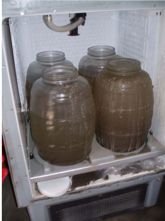
Figure 21: Wet weather composite sample collected at Receiving Water Station W-4 during December 2006 (Event 1) showing high suspended solids content
