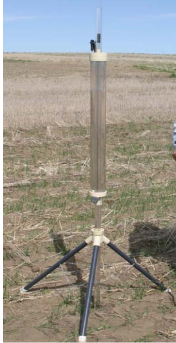
Figure C-3: Guelph Permeameter for Shallow Borehole Permeability
