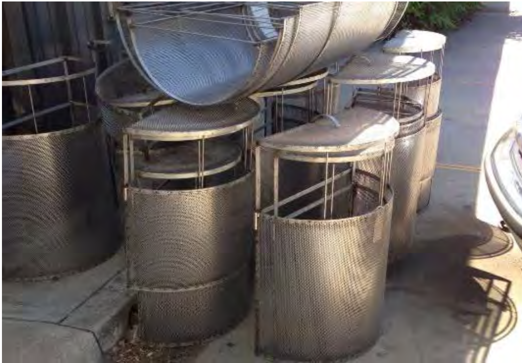
Trash excluders ready for installation
