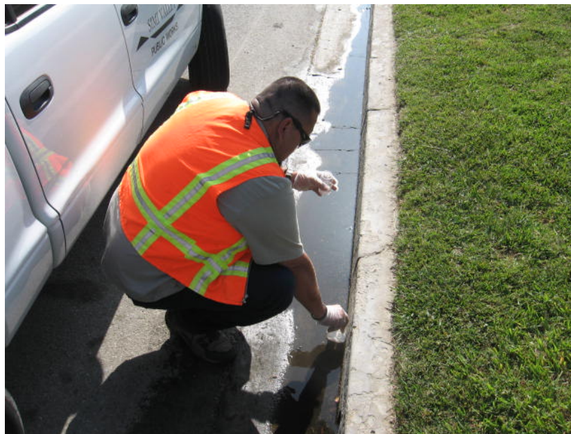
An inspector takes samples of a suspected illicit discharge
