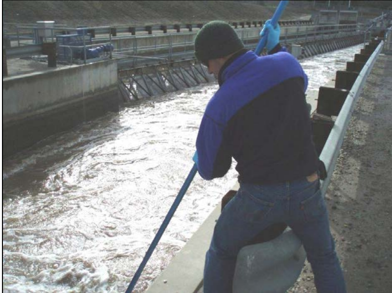
Figure 9-7. Grab Sampling Using Extended-Reach Swing Sampler
