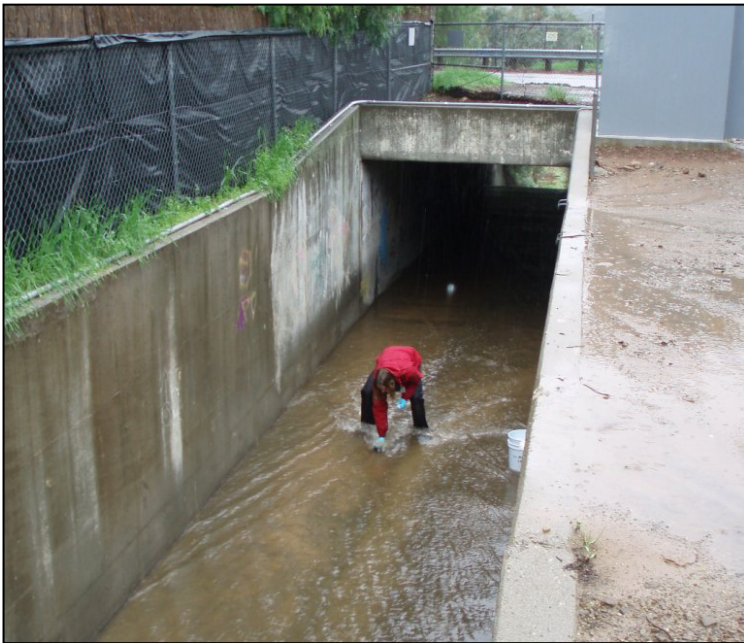
Figure 9-9-6. Grab Sampling at Mid-Stream, Mid-Depth
