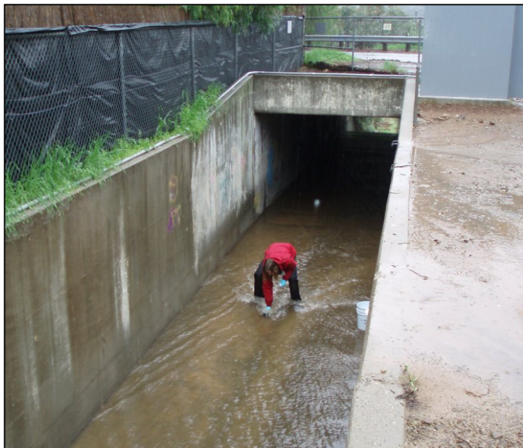
Figure 9-9-6. Grab Sampling at Mid-Stream, Mid-Depth
