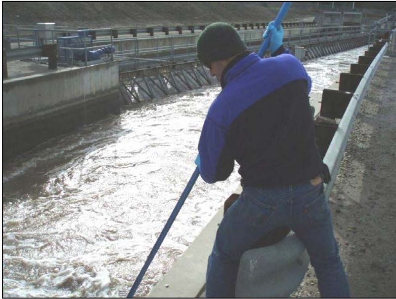
Figure 9-7. Grab Sampling Using Extended-Reach Swing Sampler
