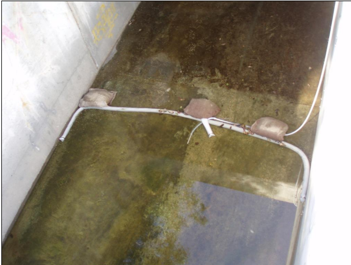
Figure 9-8. Typical Wet-Season, Dry-Weather Sampling Configuration
