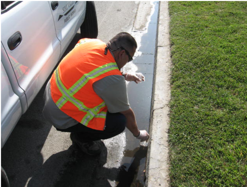
An inspector takes samples of a suspected illicit discharge
