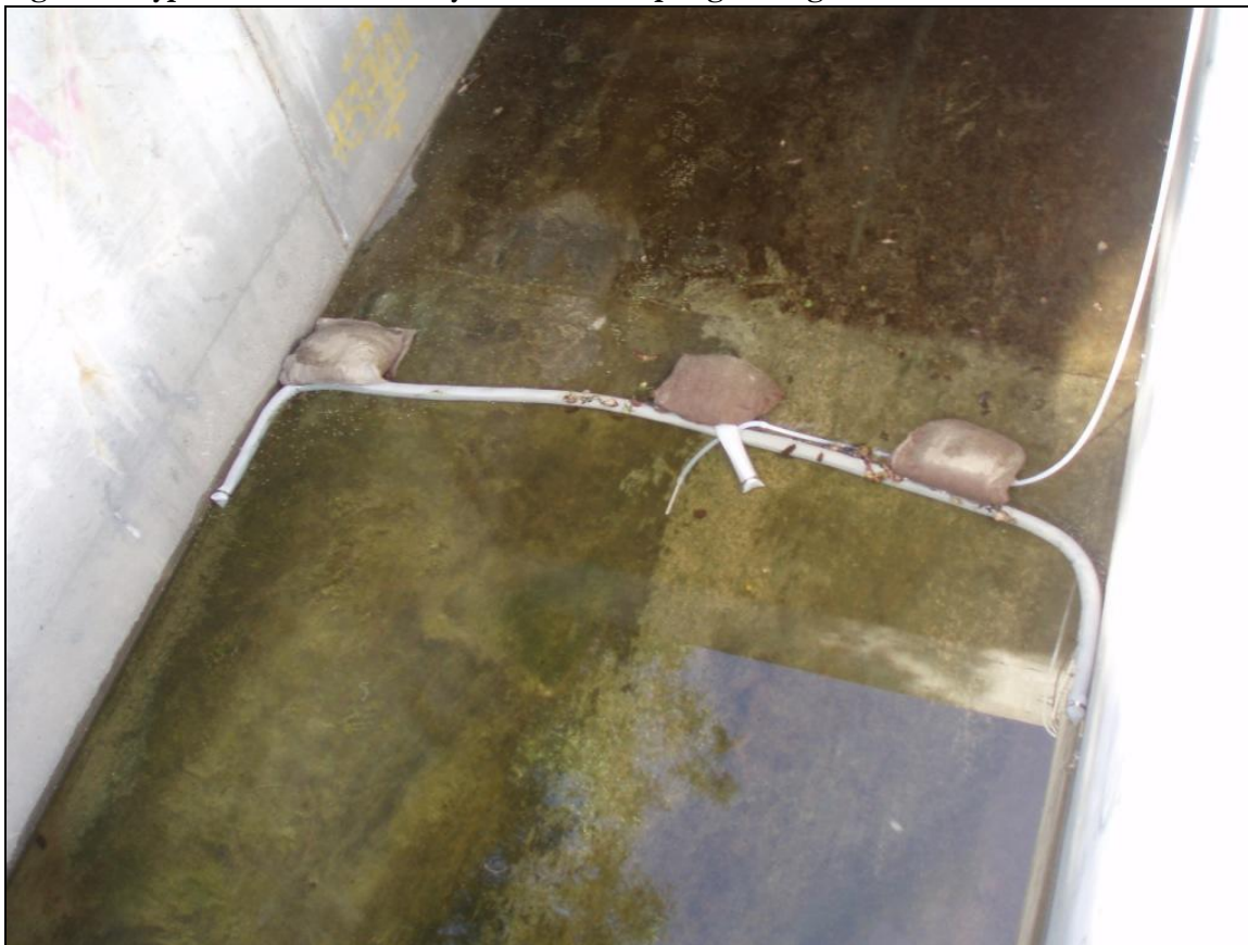
Figure 8. Typical Wet-Season, Dry-Weather Sampling Configuration
