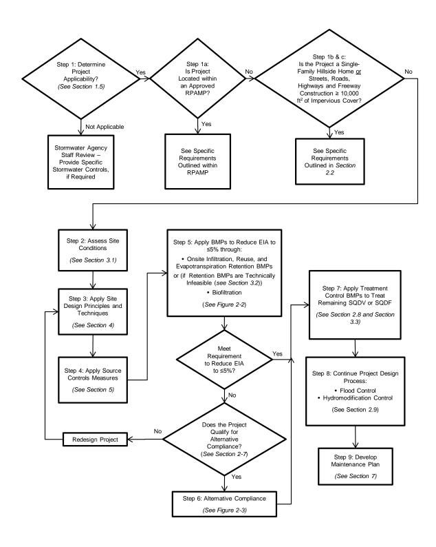
Figure 2-1: Stormwater Management Control Measures Design Decision Flowchart
