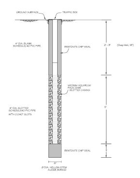
Figure C-4: Falling-Head Permeameter for Deep Borehole Permeability
