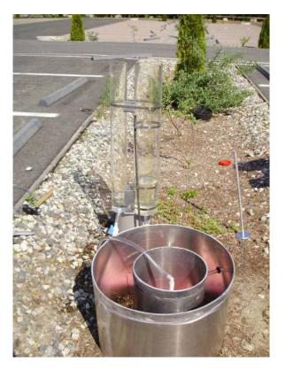
Figure C-2: Double Ring Infiltrometer
