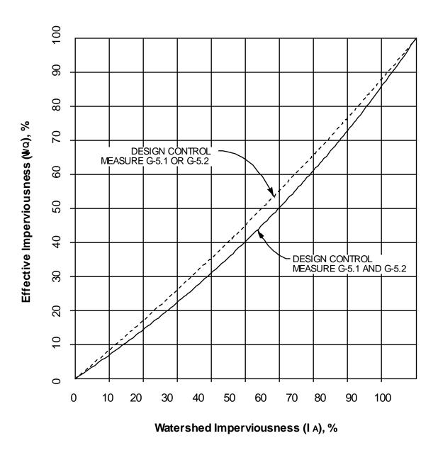
G-5.1: TURF BUFFER G-5.2: GRASS-LINED CHANNEL ADAPTED FROMURBAN STORMDRAIN ORTIERIA MANUAL VOL: 3-BESTMANAGEMENTPRACTICES, URBAN DRAINAGE AND FLOOD CONTROL DISTRICT, 11/99
