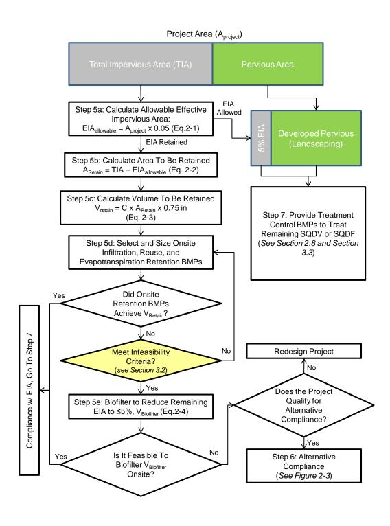
Figure 2-2: Apply BMPs to Reduce EIA to ≤5% Process Flow Chart
