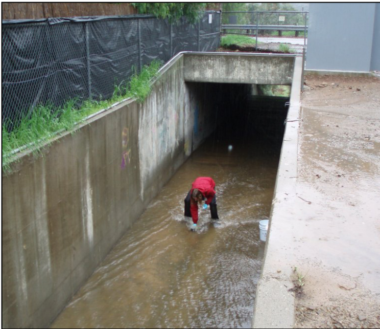
Figure 9-9-6. Grab Sampling at Mid-Stream, Mid-Depth
