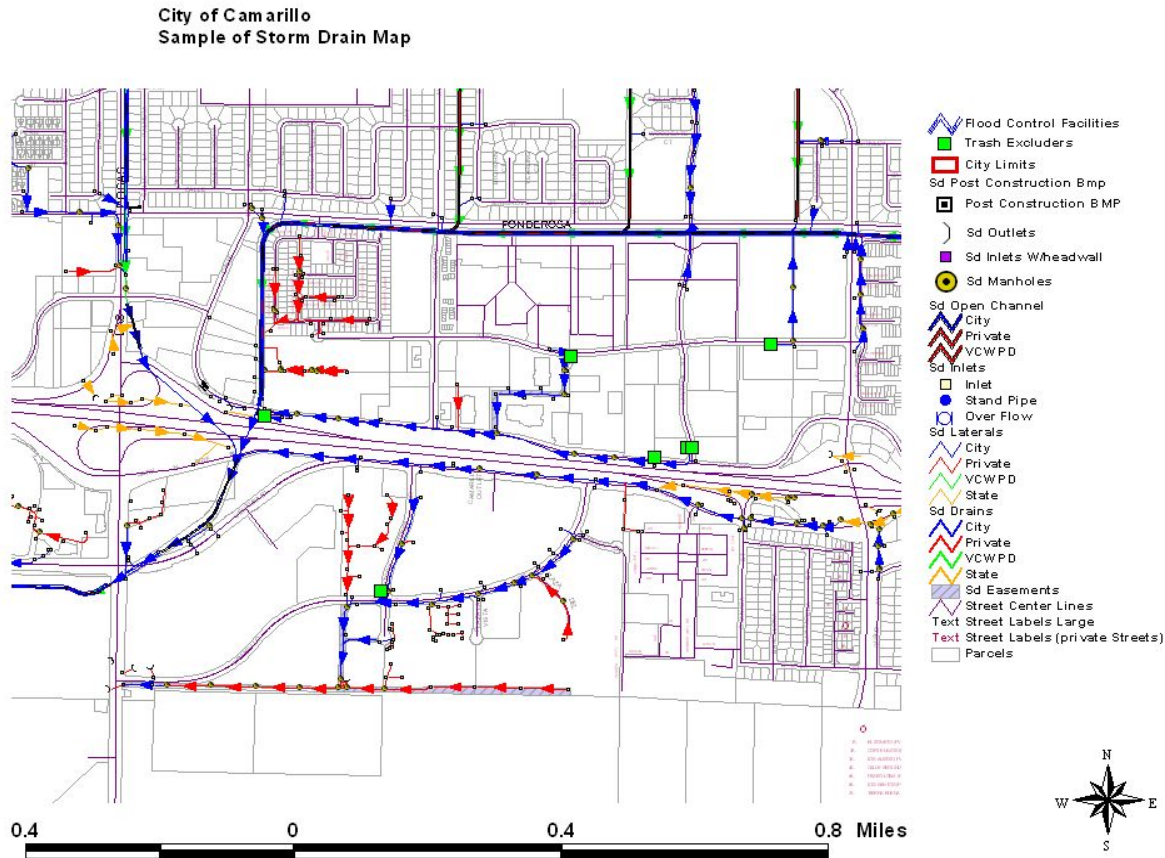
Figure 7-3 Example of Storm Drain Map
