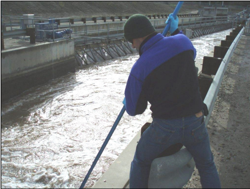
Figure 9-7. Grab Sampling Using Extended-Reach Swing Sampler
