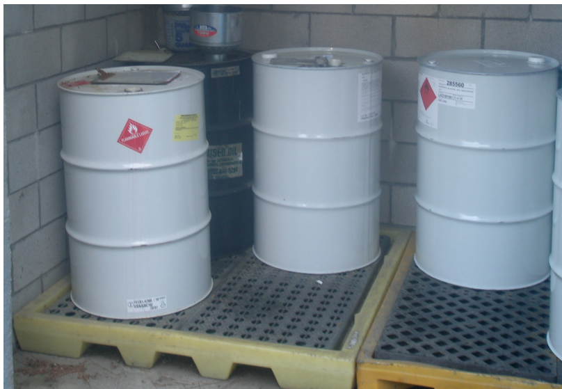
Materials stored with secondary containment
