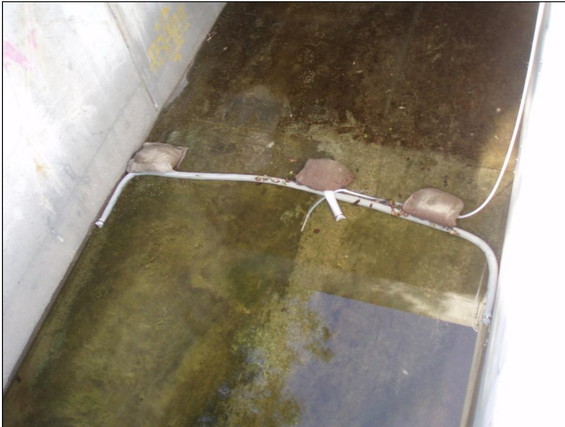
Figure 9-8. Typical Wet-Season, Dry-Weather Sampling Configuration
