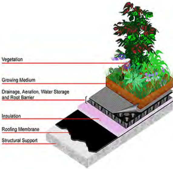
Exhibit B: Green Roof Schematic Courtesy of American Wick
