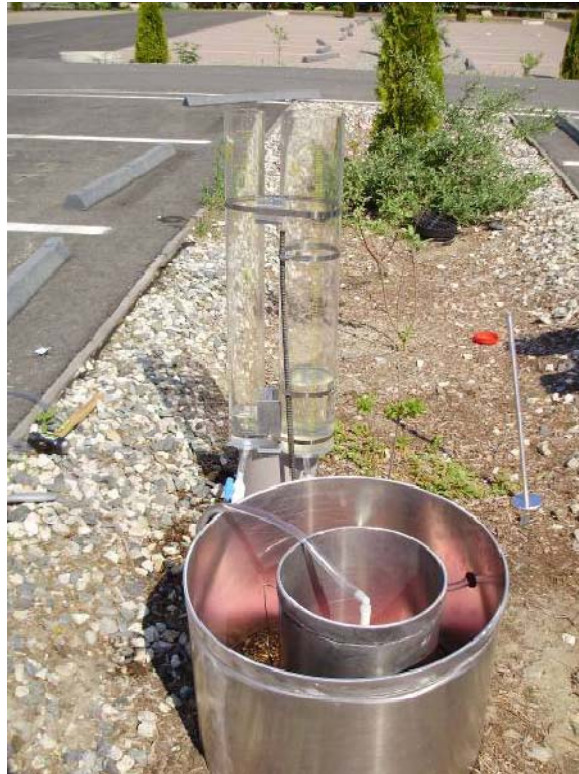
Figure C-2: Double Ring Infiltrometer
