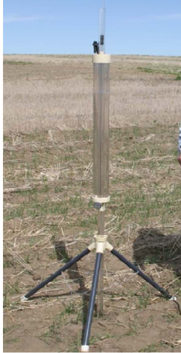
Figure C-3: Guelph Permeameter for Shallow Borehole Permeability
