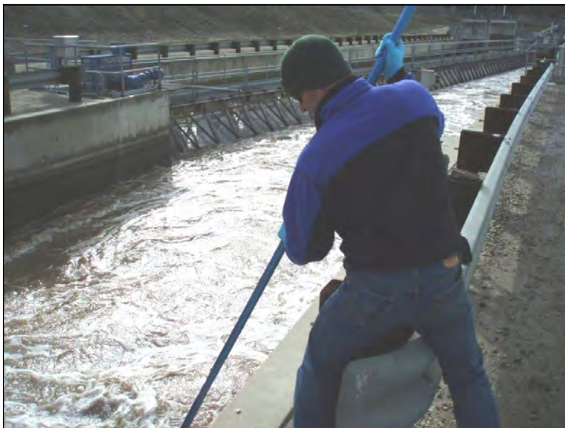
Figure 1-6. Grab Sampling Using Extended-Reach Swing Sampler
