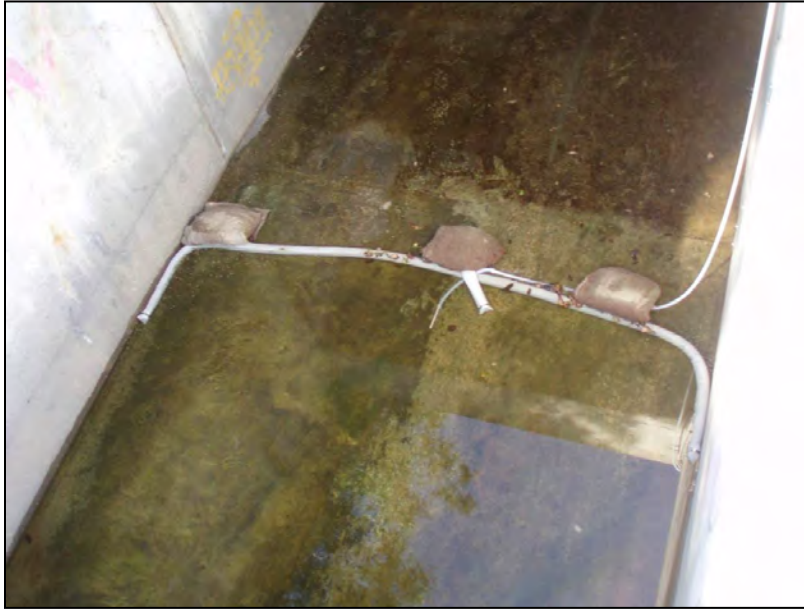
Figure 1-7. Typical Wet-Season, Dry-Weather Sampling Configuration
