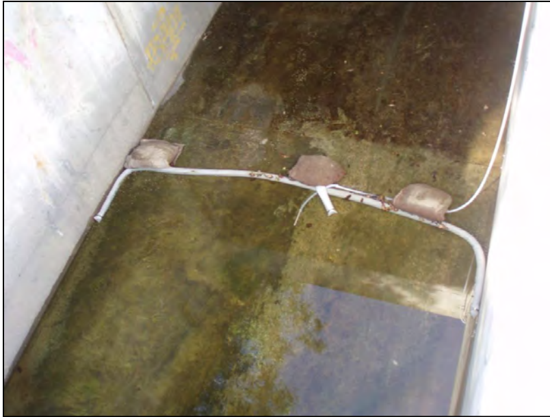
Figure 9-8. Typical Wet-Season, Dry-Weather Sampling Configuration
