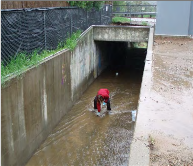
Figure 9-6. Grab Sampling at Mid-Stream, Mid-Depth
