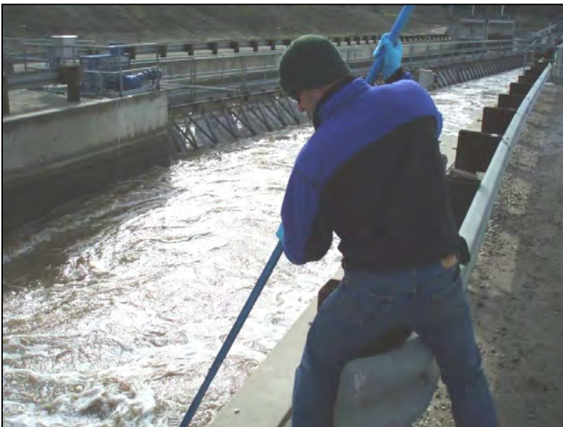
Figure 9-7. Grab Sampling Using Extended-Reach Swing Sampler
