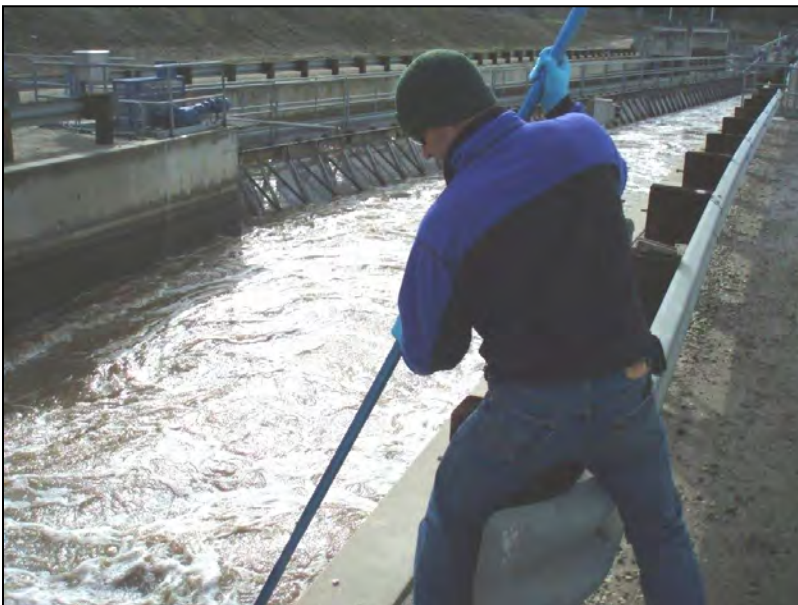
Figure 9-7. Grab Sampling Using Extended-Reach Swing Sampler
