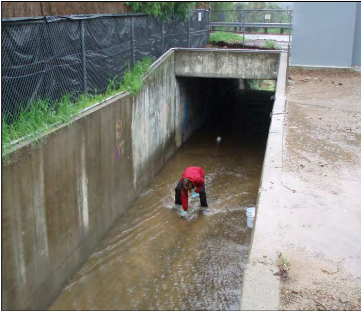
Figure 9-6. Grab Sampling at Mid-Stream, Mid-Depth
