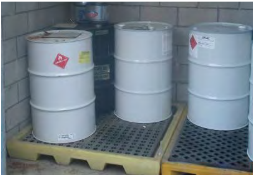
Materials stored in a covered shed with secondary containment
