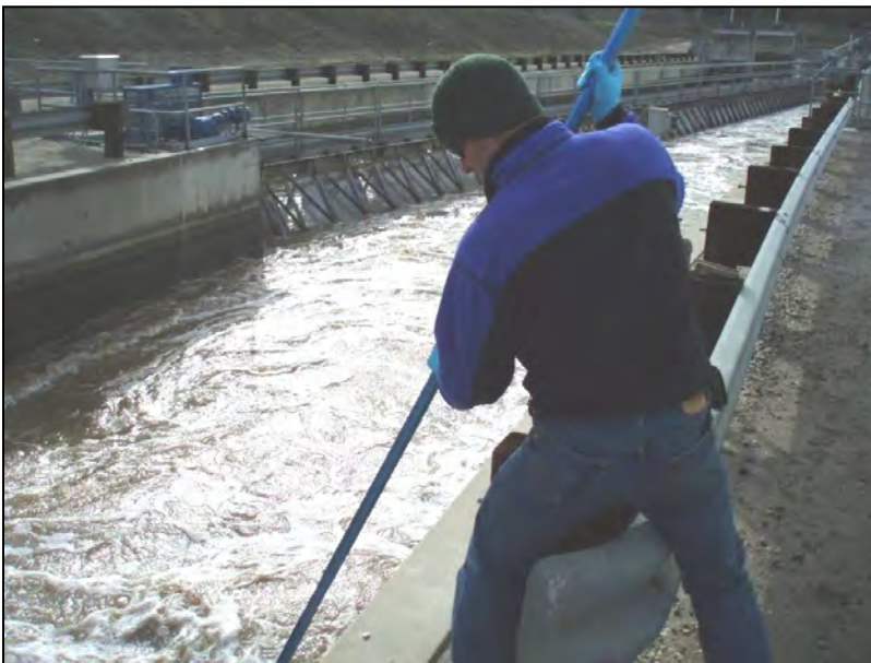
Figure 9-7. Grab Sampling Using Extended-Reach Swing Sampler
