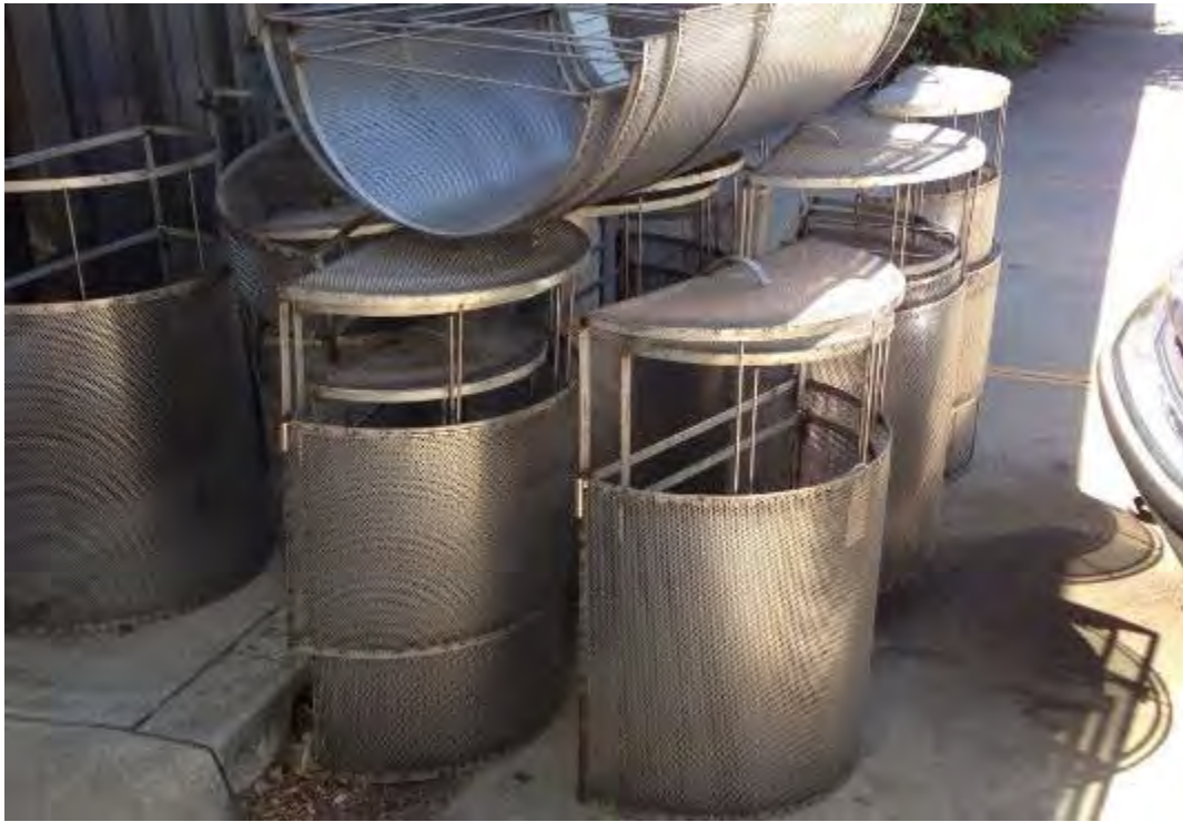
Trash excluders ready for installation
