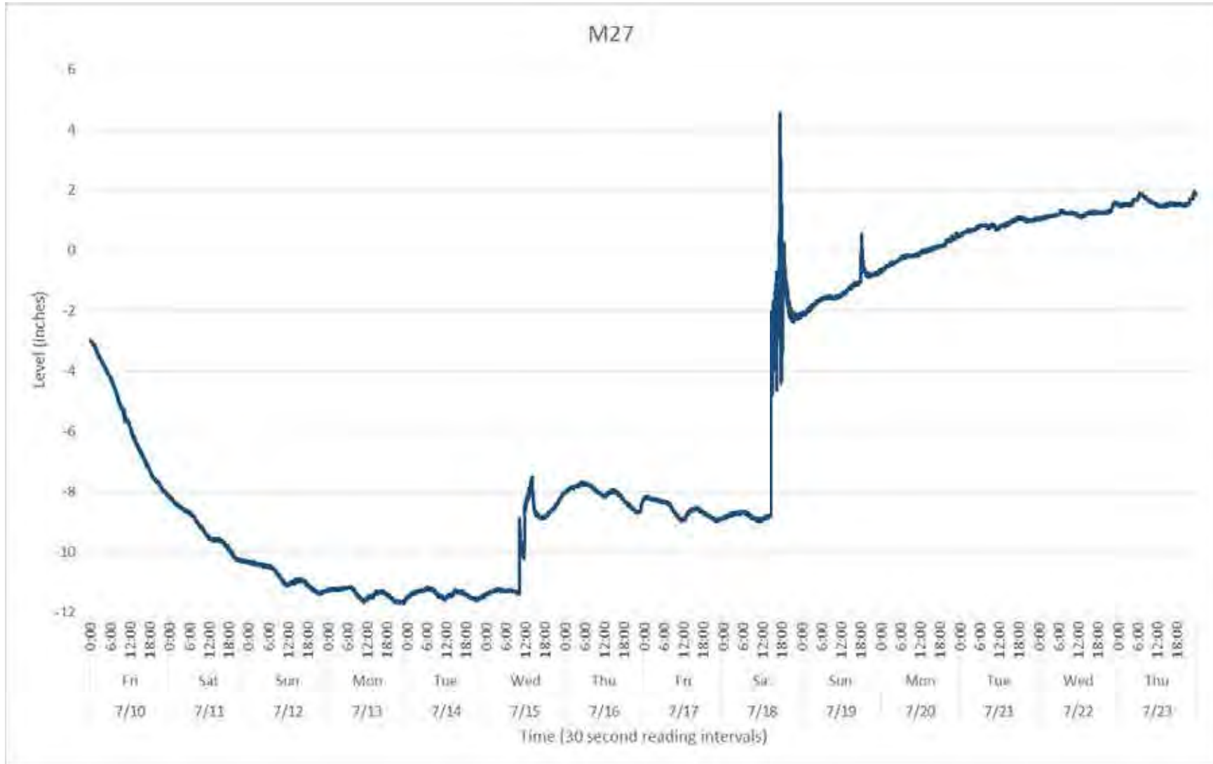
Figure E-8. Level logger data plot for outfall M27. *Data indicates the level logger malfunctioned during deployment.
