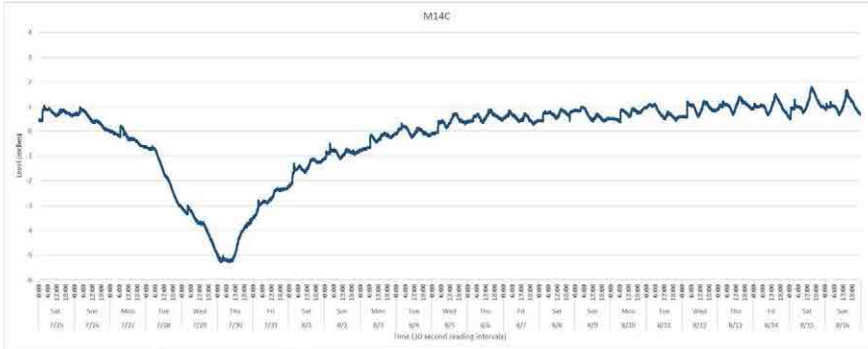
Figure E-5. Level logger data plot for outfall M14C. *Data indicates the level logger malfunctioned during deployment.
