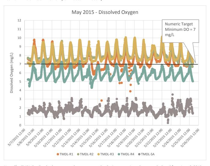
Note: The TMDL-Est dissolved oxygen results are suspected to be incorrect. A sonde was re-deployed from June 6, 2015 to June 15, 2015 at TMDL-Est to log dissolved oxygen (Figure 7). The TMDL-Est data is excluded from this chart but is included in the electronic attachments to this report.
