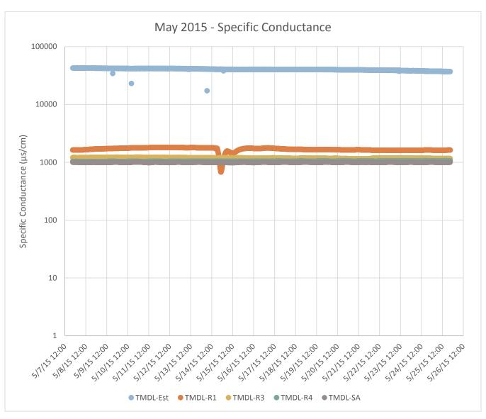
Note: The TMDL-R2 results for specific conductance are highly suspect, as the values decreased noticeably from the time of deployment and dropped well below both the expected range and the values measured by the upstream and downstream sondes. Fouling is suspected. The data is excluded from this chart but is included in the electronic attachments to this report. Specific conductance is not a required continuous monitoring parameter so the sonde was not re-deployed for this quarter.
