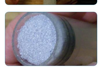
Before each sampling event, attach a fresh circular scrubbing pad to the end of the plunger. This is a head-on view of the plunger, with the scrubbing pad circle attached.
