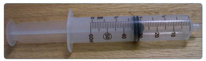
You will need a 60-mL plastic syringe for each sampler you want to make. Remove the plunger and saw the conical end off the plastic syringe, then sand the bottom so it is flat all the way around and fits tightly against a flat surface.
