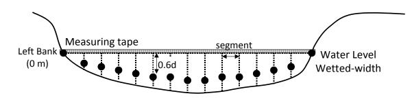
Figure 9. Diagram of layout for discharge measurements under the velocity-area method showing proper positions for velocity probe (black dots).
