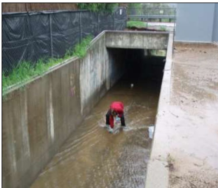
Figure 9-9-6. Grab Sampling at Mid-Stream, Mid-Depth
