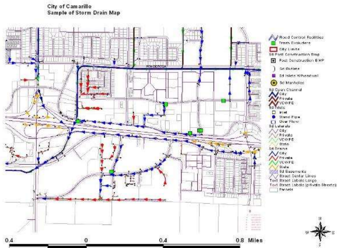
Figure 7-3 Example of Storm Drain Map
