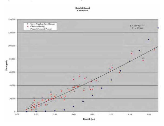
Figure 9-3. Example of Rainfall-to-Runoff Modeling Versus Actual Rainfall Events
