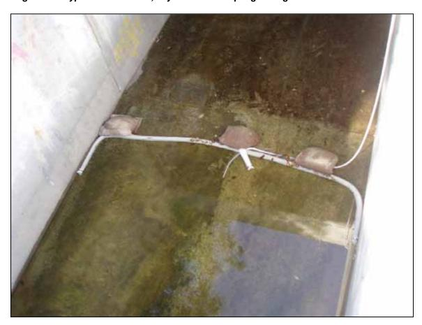
Figure 9-8. Typical Wet-Season, Dry-Weather Sampling Configuration
