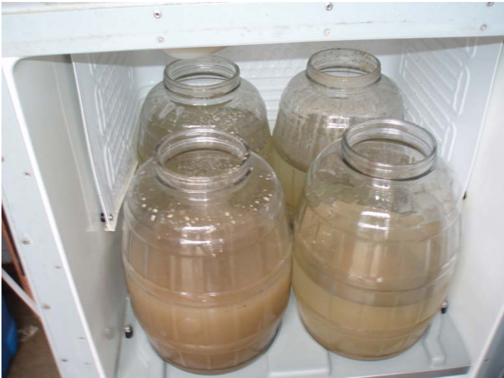
Figure 15: Wet weather composite sample collected at Mass Emission Station ME-SCR during February 2009 showing high suspended solids content
