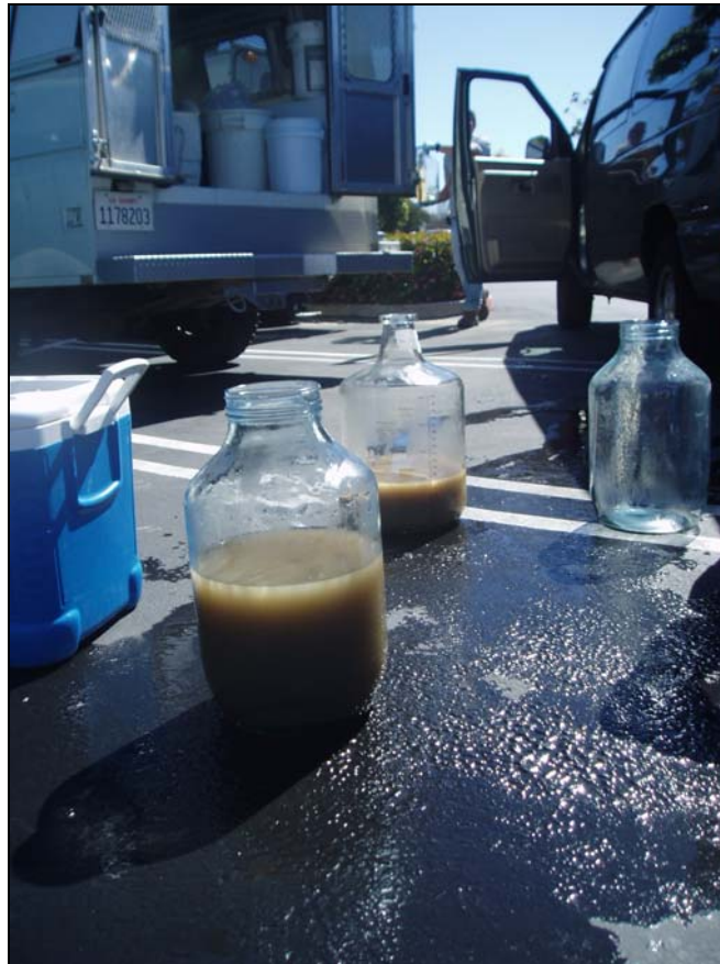
Figure 24: Wet weather composite sample collected at Mass Emission Station ME-CC during February 2006 (Event 4) showing high suspended solids content
