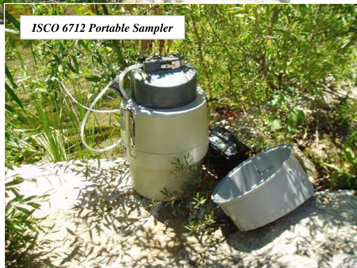
Figure 9-19: Newly sited Mass Emission Station ME-VR2 showing ISCO 6712 portable sampler used to monitor 2004-2005 dry weather events in the Ventura River
