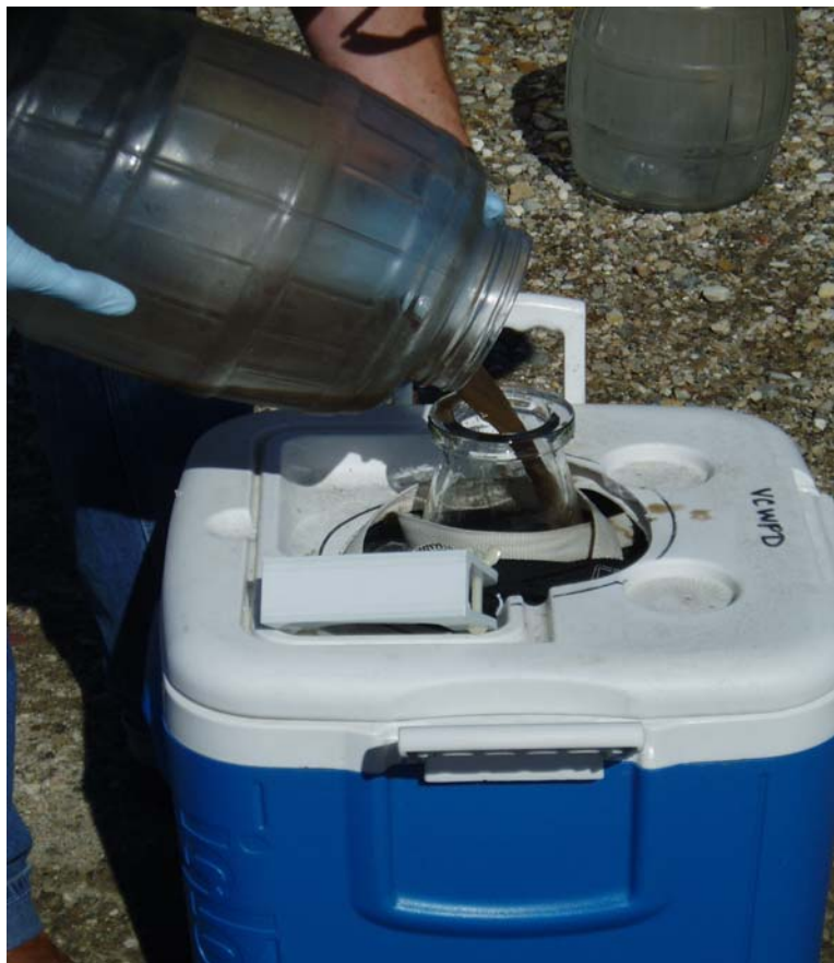
Figure 9-35: Wet weather composite sample collected at Mass Emission Station ME-SCR during January 2005 (Event 4) showing high suspended solids content
