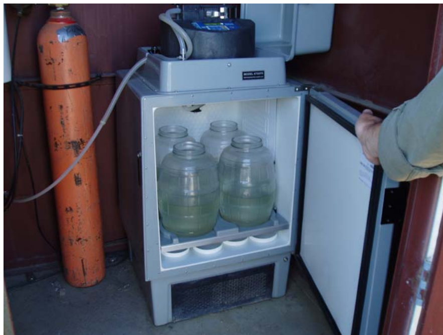
Figure 9-20: ISCO 6700FR Refrigerated Sampler installed at Mass Emission Station ME-SCR
